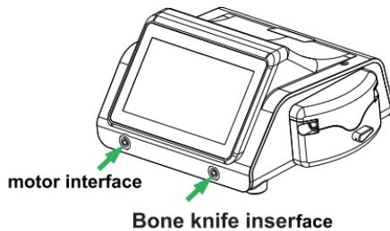
► Insert the motor plug into motor interface of the device, align the marking points and insert the plug until it locks.
