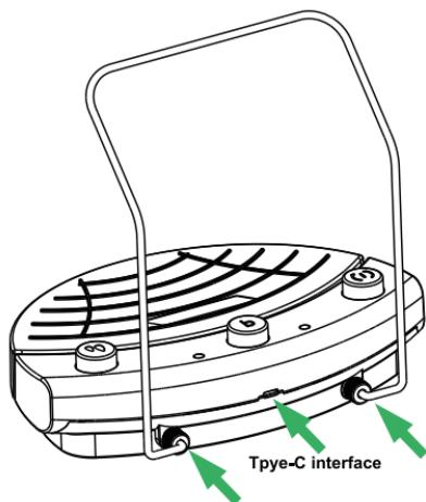
► Insert the pedal handle into the groove of the pedal and then tighten the nut manually.
