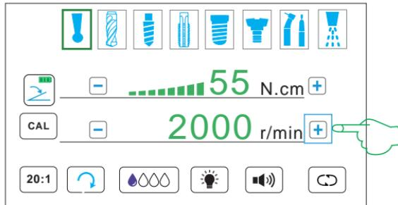
► Press "+" or "-" to adjust the highest speed within the specified range.
